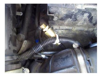
The top pipe and electrical connector should remain on the EBV. Use a bit of pipe to block off the two bottom pipes. I've used a cable tie as well to ensure it stays put. Then screw the EBV back onto its mount.
