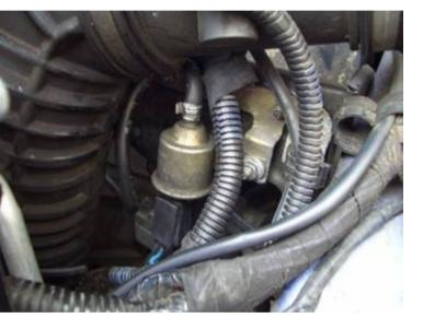
Use a cable tie to hold the PRV in position so that you can still adjust it, the cables aren't bent, and it doesn't move around.
